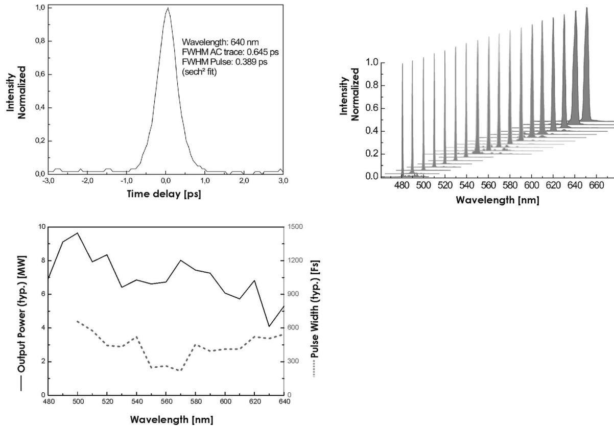
**Figure 17** Typical pulse characteristics, emission spectra and power distribution of the tunable FemtoFiber® pro TVIS system
