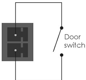
**Figure 23** Interlock connector
