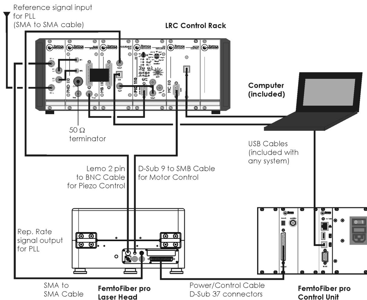
**Figure 56** Connections for FemtoFiber<sup>®</sup> pro LRC-option
