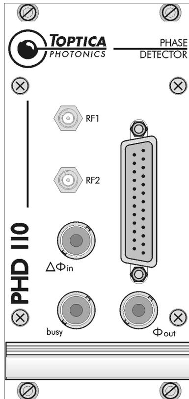
**Figure 58** Front panel of the PHD 110 module
