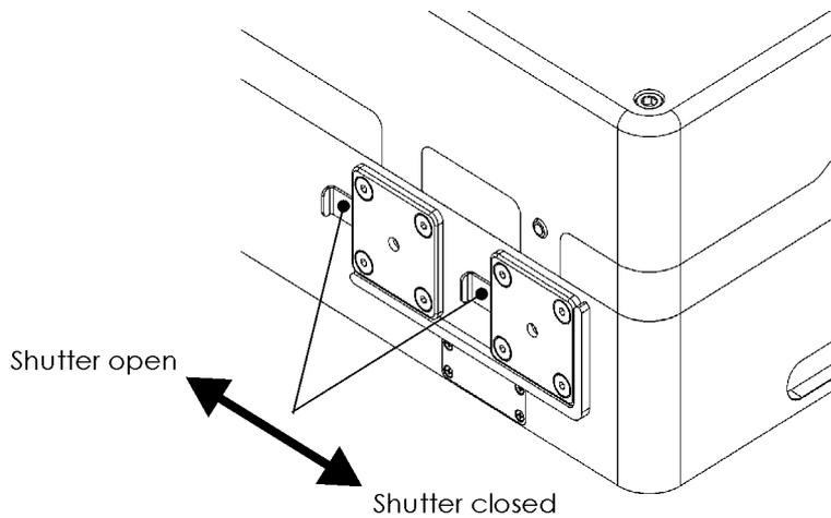
**Figure 24** FemtoFiber® pro laser head aperture shutter
