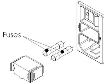
**Figure 25** Fuses at FemtoFiber® pro control unit connector block
