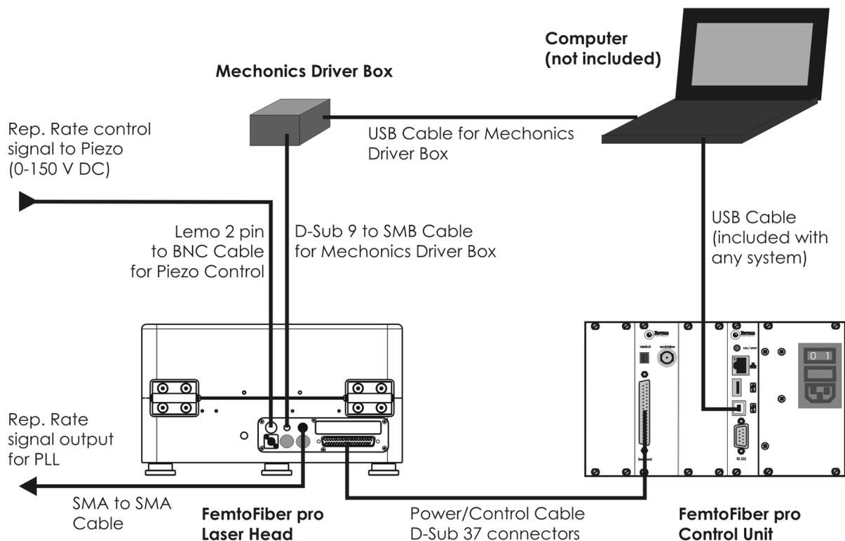
**Figure 55** Connections for FemtoFiber<sup>®</sup> pro VAR-option
