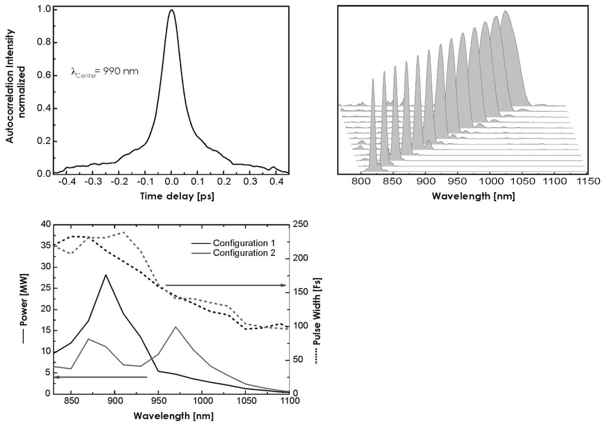
**Figure 19** Typical pulse characteristics, emission spectra and power distribution of the tunable FemtoFiber® pro TNIR system, available in two configurations
