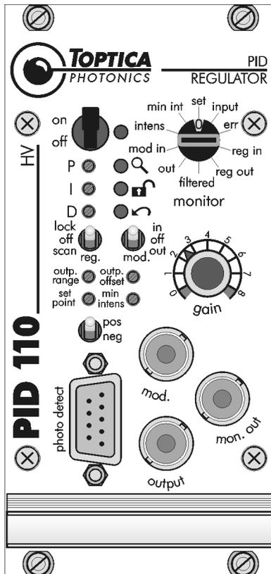
Figure 60 Front panel of the PID 110 module
