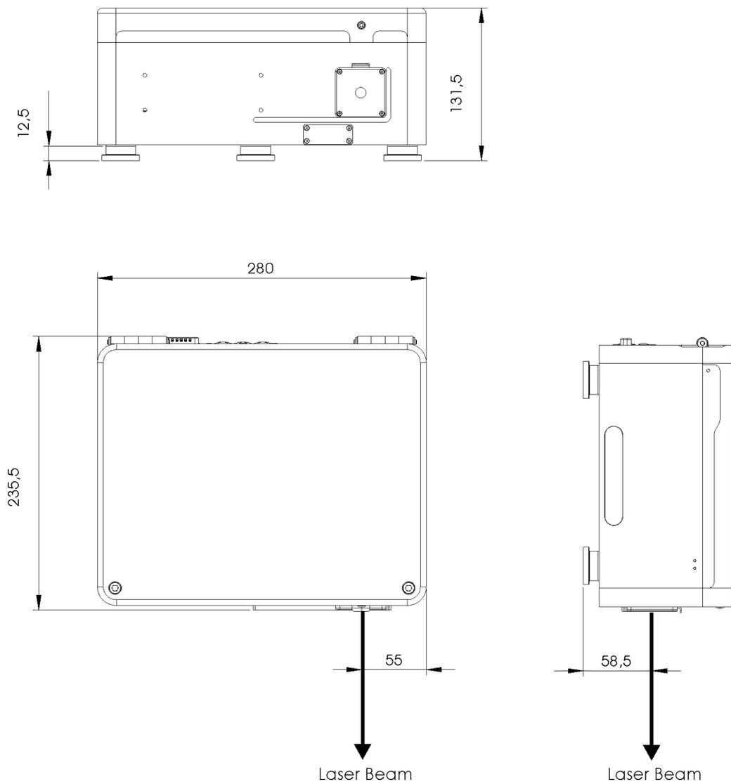
**Figure 68** FemtoFiber<sup>®</sup> pro laser head main dimensions and apertures (IRS-II/SCYb)
