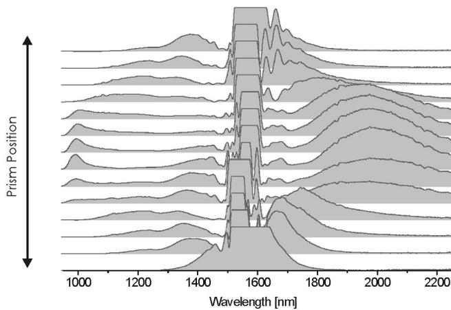
**Figure 13** FemtoFiber® pro SCIR continuum in dependence of prism position
