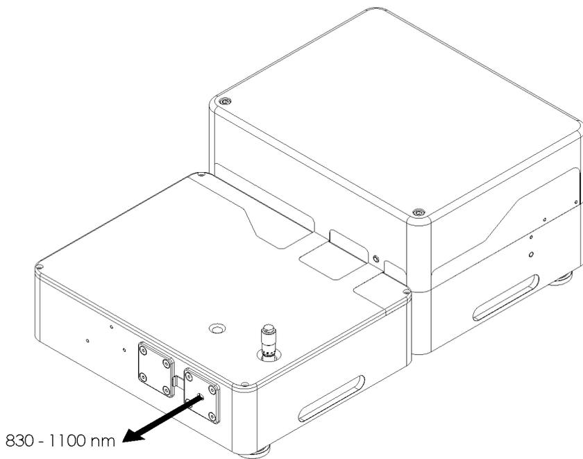
**Figure 18** FemtoFiber® pro TNIR laser beam
