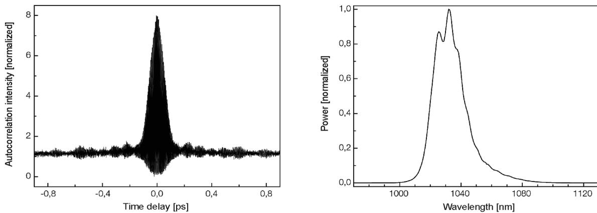
**Figure 11** Typical pulse characteristics and emission spectrum of FemtoFiber® pro SCYb
