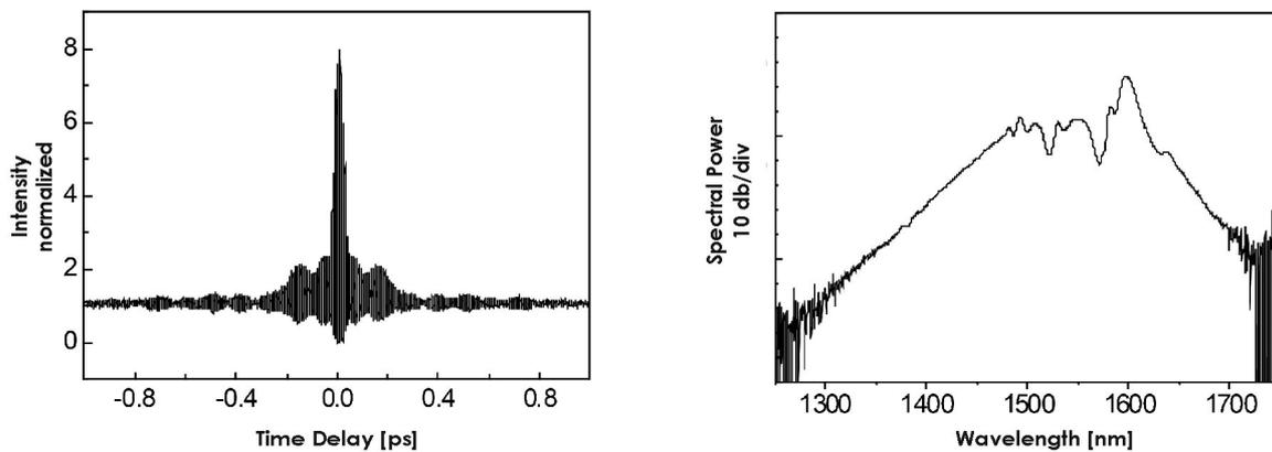
**Figure 6** Typical Pulse characteristics and emission spectrum of FemtoFiber<sup>®</sup> pro IRS-II
