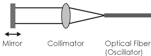
**Figure 21** Optical setup of the VAR-option
