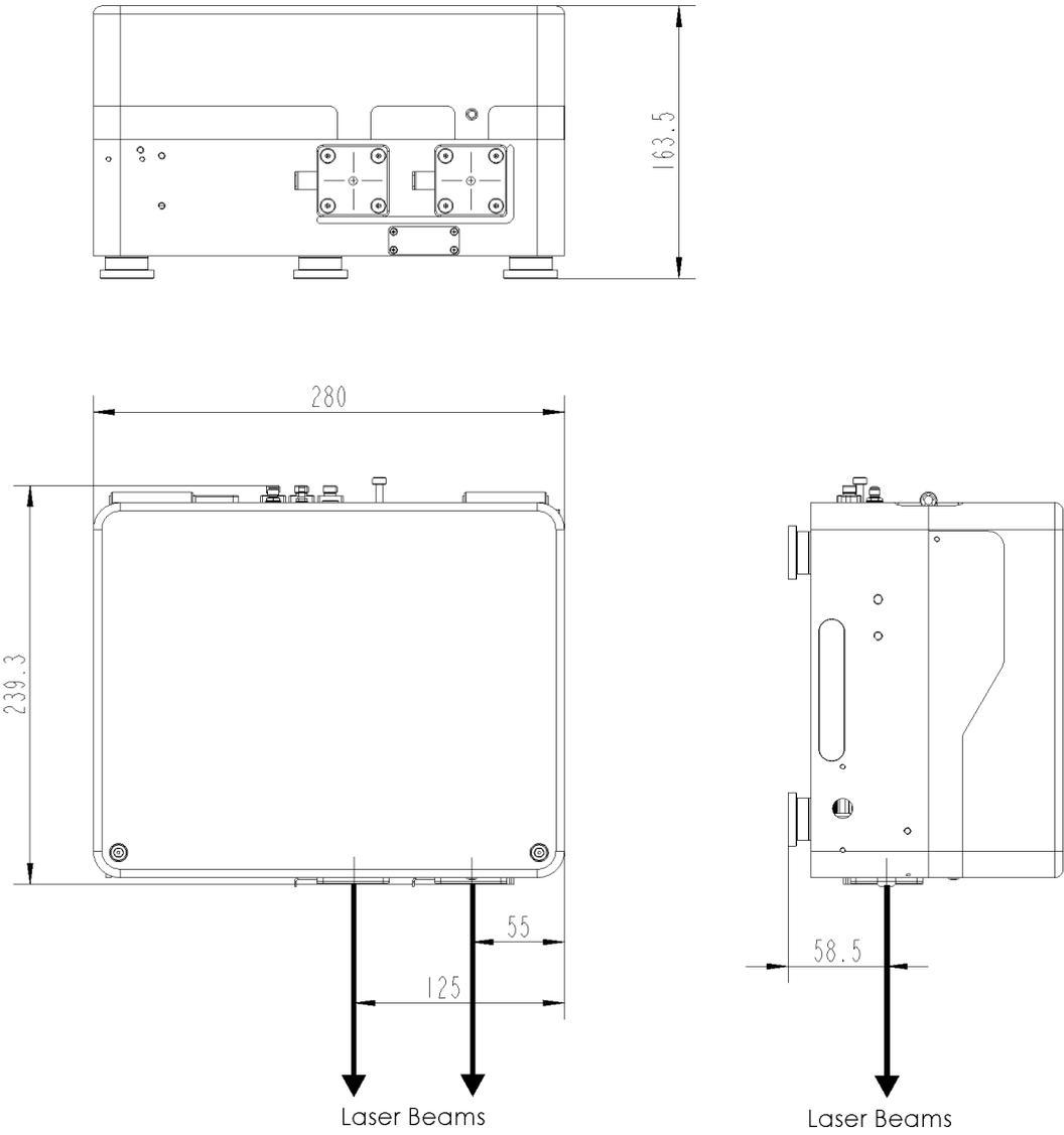
**Figure 67** FemtoFiber® pro laser head main dimensions and apertures (IR/NIR/SCIR) (all possible apertures shown)
