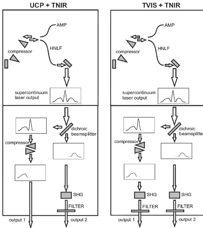
**Figure 22** Schematic setup for TNIR-option (UCP, TVIS)
