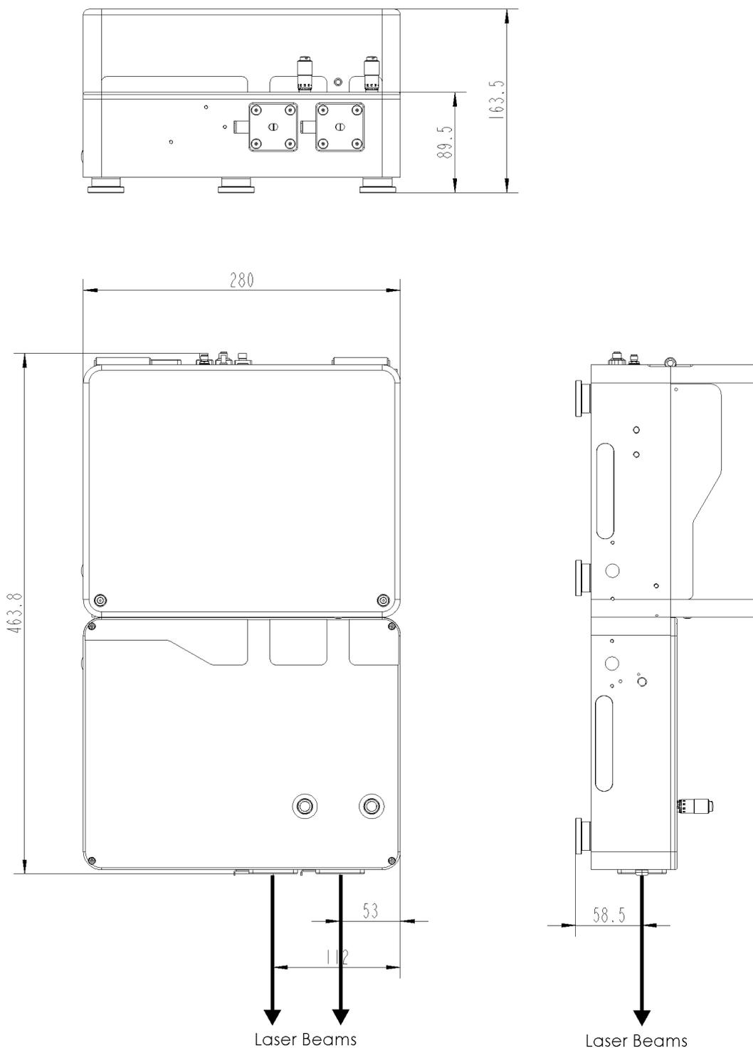
**Figure 69** FemtoFiber® pro laser head main dimensions and apertures (UCP/TVIS/TNIR) (all possible apertures shown)
