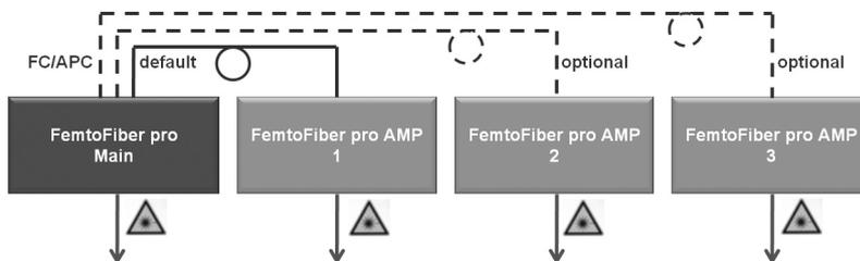
**Figure 20** FemtoFiber® pro main (master) system with 3 AMP (slave) systems
