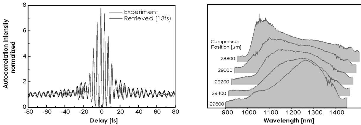
**Figure 15** Typical Pulse characteristics and emission spectrum of FemtoFiber® pro UCP
