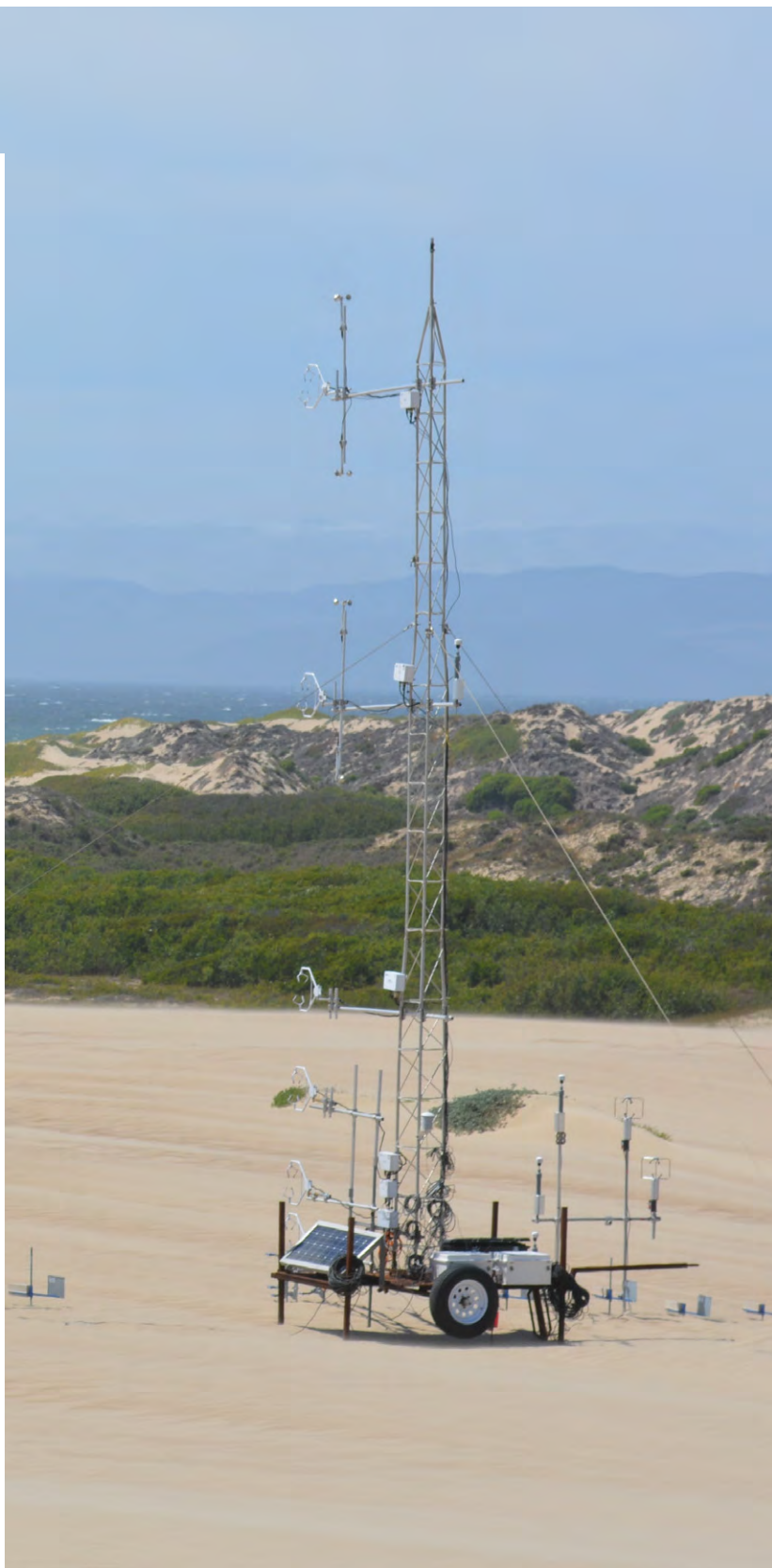
Field setup showing the 10-meter tower with sonic anemometers.
