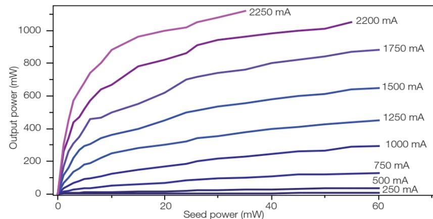
Typical saturation behavior of tapered amplifier chips at different amplifier currents (seed power levels exceeding 40 mW are not recommended).
