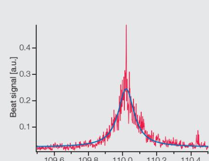
Linewidth measurement of DL 100 with delayed self-heterodyne beat setup (delay 5 μs). The resulting linewidth is below 100 kHz.
