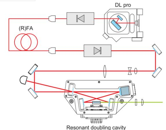
The versatility of TOPTICA's lasers allows for straight forward implementation of (Raman) fiber amplifiers.
