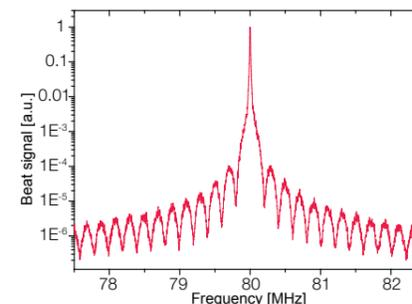
A self-heterodyne linewidth measurement shows a short-term linewidth of a free-running DLC DL pro (narrow linewidth option) of only 5 kHz.
