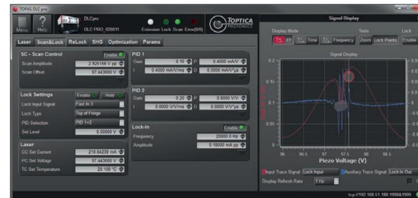
Convenient laser control via remote PC-operation: Users can easily set all relevant parameters via the graphical user interface.
