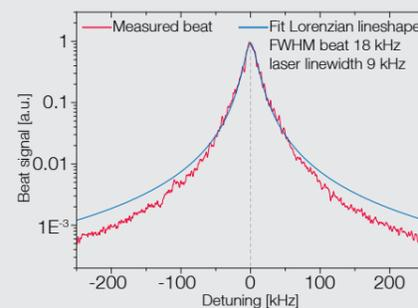
Measured beat signal of two free-running DL pro at 1160 nm. 100 scans with sweep times of 50 ms have been averaged. The two laser systems are of the same built and contribute equally to the residual noise.
