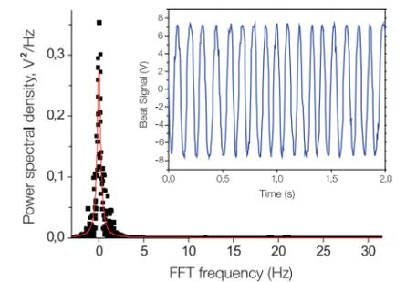
Beat measurement of two independent ECDLs locked to two high-finesse ULE cavities, one of them using FALC 110. The beat width was less than 0.5 Hz over 8 s. The inset shows the phase stability of the beat note filtered with a 100 Hz low-pass filter (J. Alnis, MPQ Garching).
