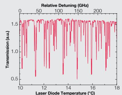
Absorption spectrum of iodine, recorded with a thermally tuned DFB pro laser at 633 nm. The scan in the figure covers a range of approx. 250 GHz.
