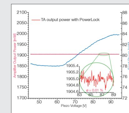
DLC TA pro system master and amplifier powers with PowerLock during a 10 Hz piezo scan. While the master fluctuates approx. 8%, the TA output is stable ( $\sigma=0,01\%$ ).
