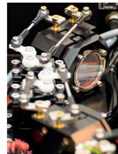
With AutoAlign, the user starts optimization of the beam alignment with one simple click. Built-in servos and digital intelligence do the rest of the job.
