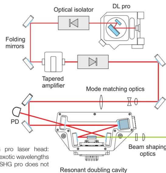
Schematic of the TA-SHG pro laser head: High power at common and exotic wavelengths (Medium-power version DL-SHG pro does not include the TA section.).
