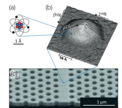
The CTL is ideally suited to investigate microcavities. Such cavities are useful for sensing applications, investigating quantum-mechanical coupling, and to create microscopic frequency combs.
