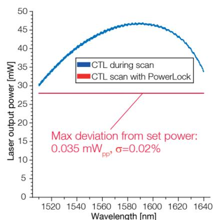
Output power as a function of the wavelength of the CTL 1550. The smooth power variation of only ~20 % over the whole specified tuning range can be reduced to below 0.1 % with PowerLock.
