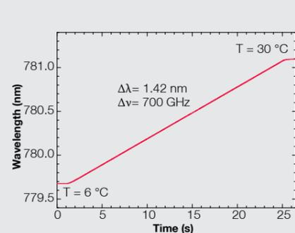
“Wide scan” of a DFB pro laser at 780 nm: A temperature sweep from 3 °C to 30 °C changes the frequency by 700 GHz.
