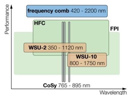
Comparison of frequency references. The performance represents aspects like accuracy, repeatability or achievable linewidth. Shown are: Frequency comb (DFC) wavelength meters (WSU), spectroscopy cells (CoSy), Fabry-Pérot interferometers (FPI), and high finesse cavities (HFC).
