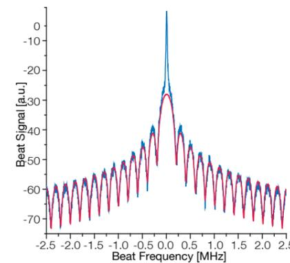
Measurement of the CTL 950 linewidth with a self-heterodyne beat experiment with a 1 km (5  $\mu$ s) delay fiber. The result is a linewidth of approximately 5 kHz.
