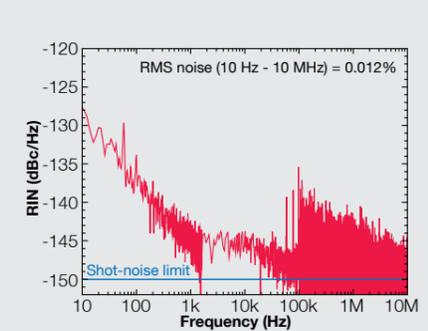
Relative intensity noise (RIN) of a DFB pro laser at 780 nm. The integrated RMS noise amounts to 0.01%.
