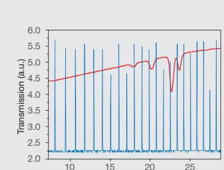
DL 100 frequency sweep over four Rb absorption lines (red). FPI transmission peaks (blue, FSR 1 GHz) are shown for reference.
