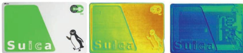
Photograph and terahertz images of a Japanese pre-paid public-transport card. The terahertz reflectivity image (middle) reproduces the look of the card. Removing the front-side reflection (right) provides an inside view of the underlying electronics.
