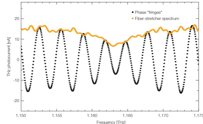
Terahertz scan across a water-vapor resonance. The black trace depicts the phase "fringes" as measured with a TeraScan 1550 system. The yellow trace shows the envelope spectrum obtained with the Phase Modulation Extension; the high frequency resolution unveils small-scale standing-wave effects in the optical path.
