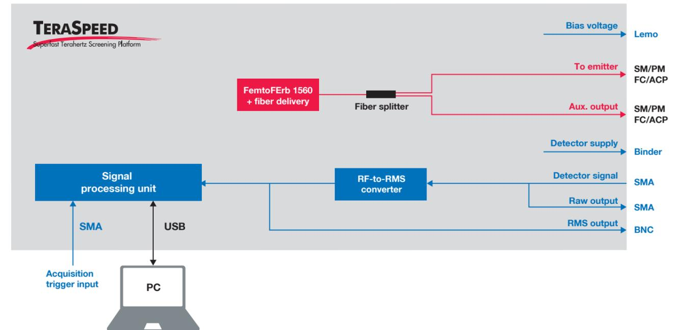
Schematic of the TeraSpeed. Red: optical signals, blue: analog signals, black: digital signals.
