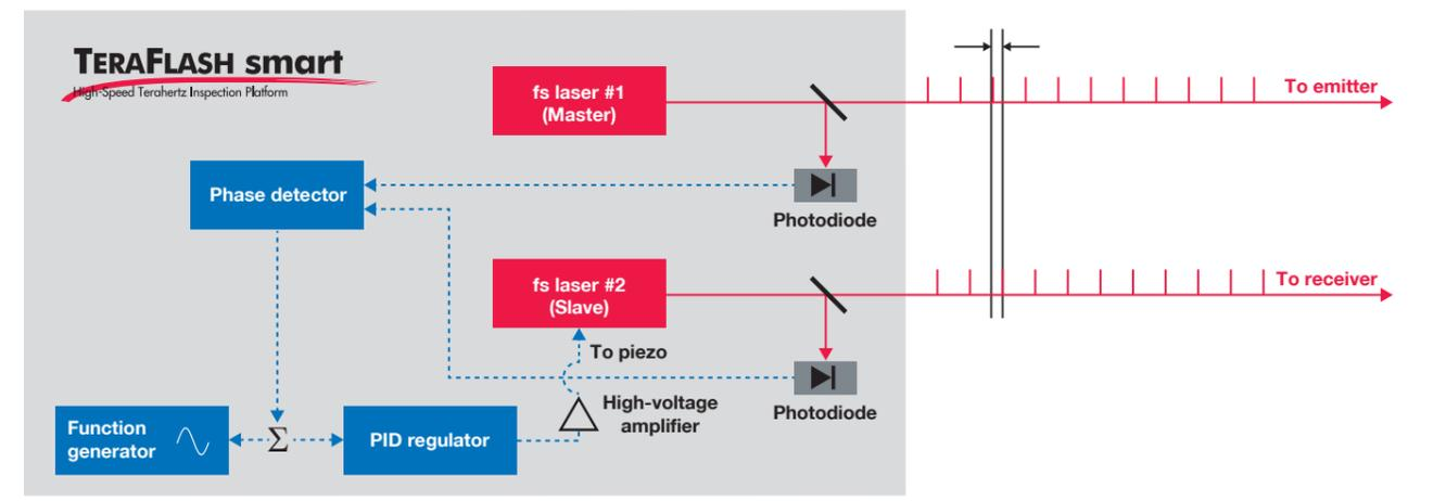
Schematic diagram of the TeraFlash smart. Blue lines depict electric signals, red lines the optical signals. The black arrows depict the momentary difference in repetition rates.
