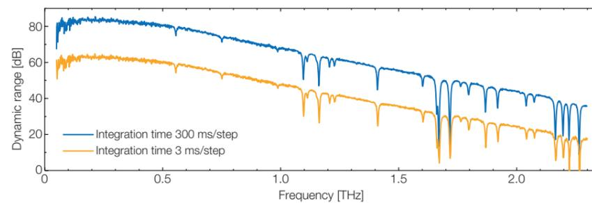
Dynamic-range spectrum of a TeraScan 780. The dips are absorption lines of water vapor.
