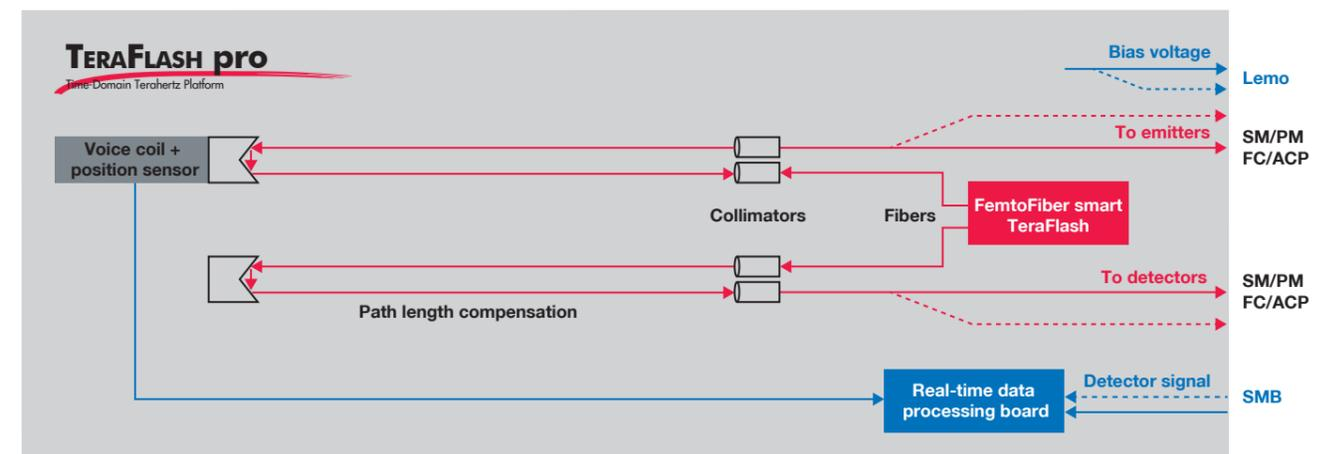
Schematic diagram of the TeraFlash pro. Blue lines depict electric signals, red lines the optical signals.
