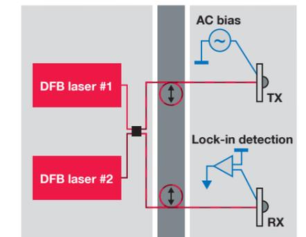
Schematic of TeraScan with Phase Modulation Extension (dark grey).
