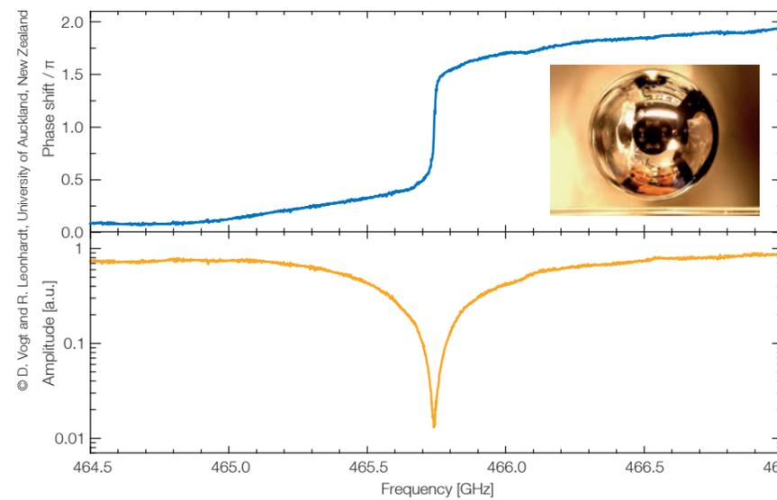
Relative phase shift (top) and amplitude spectrum (bottom) across a narrow resonance of a whispering-gallery-mode bubble-resonator made of silica glass. In the experiment, the frequency step size of a TeraScan 1550 was set to 1 MHz. The photo insert shows a sphere made of high-resistivity silicon, another material used for studying high-Q resonators.
