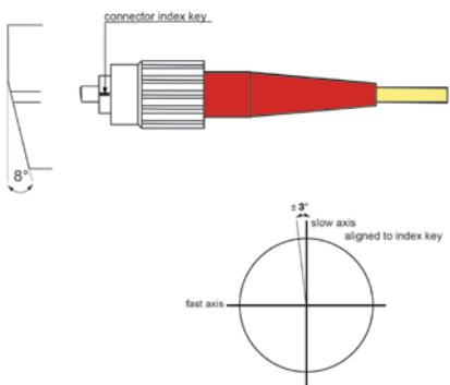
Standard fiber output connector FC/AFC and polarization orientation at fiber connector
