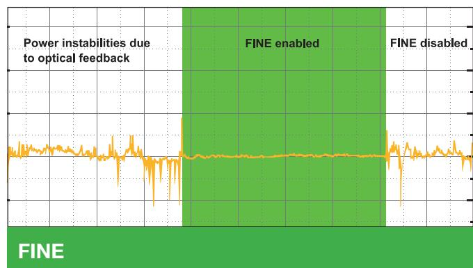
The Feedback Induced Noise Eraser FINE eliminates power instabilities and high noise levels that can be caused by back reflections into the laser. By a simple push of a button ultra-stable operation is established and the need for costly optical isolators is often eliminated.
