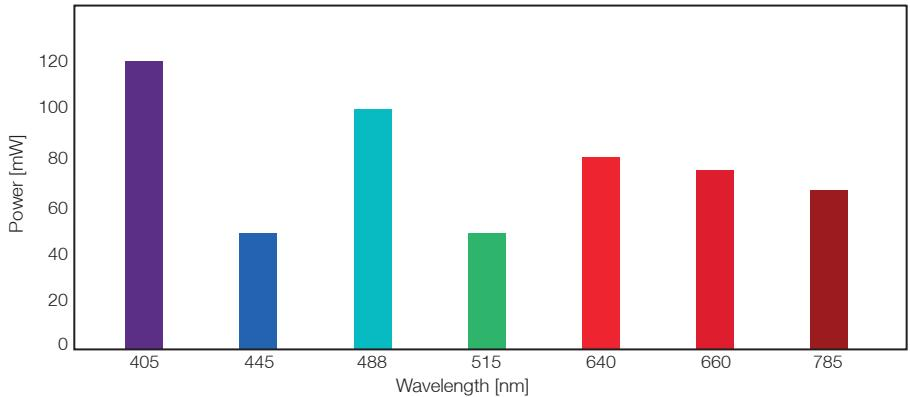
iBeam smart PT standard wavelengths with highest optical power
