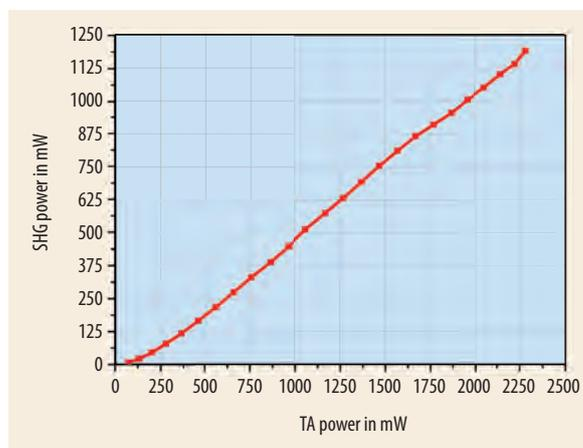
**Fig. 2** Second harmonic output power versus fundamental power for the TA-SHG pro at 626 nm
