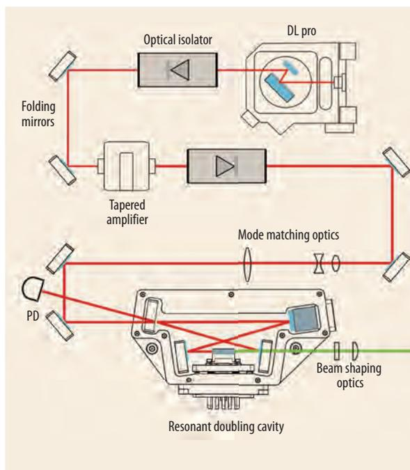
**Fig. 1** Schematic of the optical path within a TA-SHG pro: The master laser (DL pro) seeds a tapered amplifier chip. The high power output is then coupled into a resonant doubling cavity that contains the temperature stabilized nonlinear crystal.
