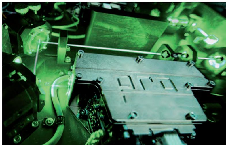
Two TA-SHG pro systems generate high output powers at 589 nm and 626 nm (above). The detailed view of the resonant frequency-doubling cavity is shown below.
