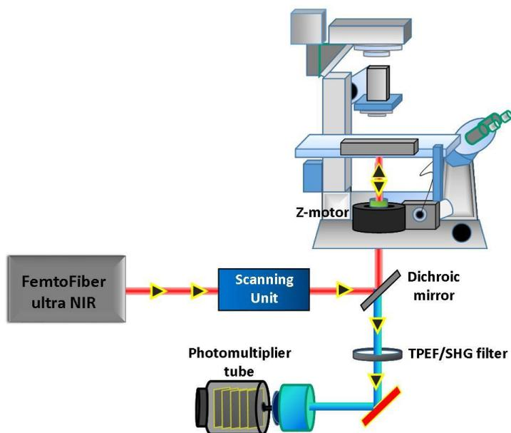
Fig. 2: Simplified schematic diagram of the multiphoton microscope.
