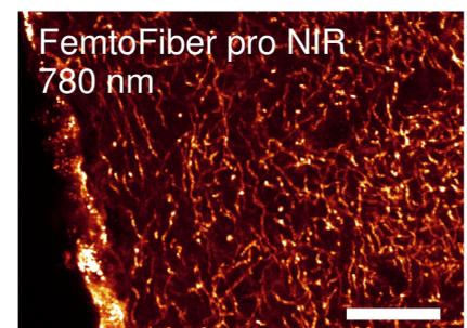
Fig 7: Same sample as in Fig. 6 but with FemtoFiber pro NIR at 780 nm, 10 mW at focal plane (scale bar 20  $\mu\text{m}$ ).
