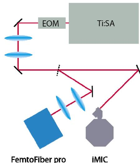
Fig. 1: Experimental setup. The Ti:Sa and the FemtoFiber pro NIR are coupled into an inverted microscope (iMic, Till Photonics). A flip-mirror (dotted line) is used to switch between the beam paths.
