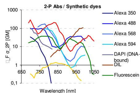
Fig. 2: 2-photon absorption spectra of typical cell and tissue stains (from [2]).
