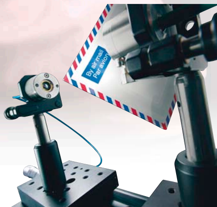
Figure 1: Terahertz spectroscopy enables the detection of hazardous substances in envelopes and parcels
