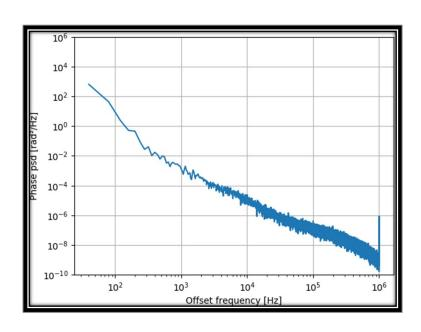
phase noise density by free running mode locked laser
