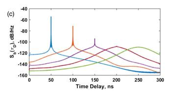
Phase-noise model for actively linearized frequency-modulated continuous-wave ladar
