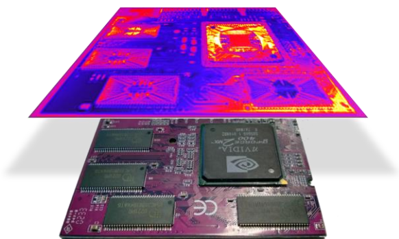
Fig. 6: Terahertz near-field reflection image of a graphic card, revealing bond wires, contact pads and other interfaces. © Protemics GmbH.
